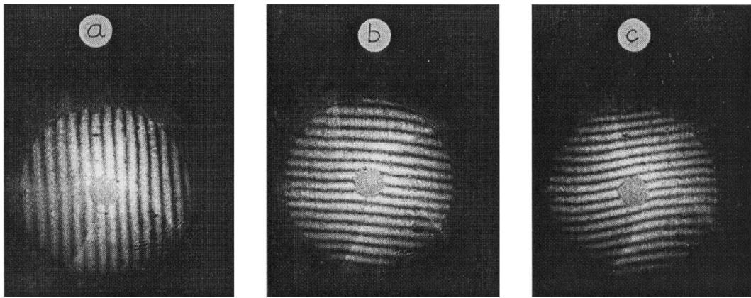
Fig. 2. Interferograms of the primary mirror. *a* and *b*: perpendicular interference fringes near the focus of the paraboloid. *c*: coma outside the region around the focal point of the paraboloid. The DOT field is small enough for no coma correction to be necessary.
